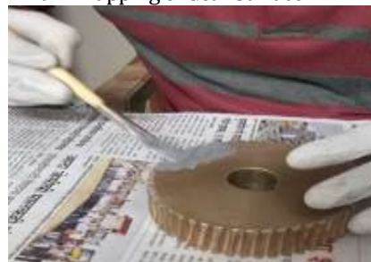
b. Application of Adhesive
