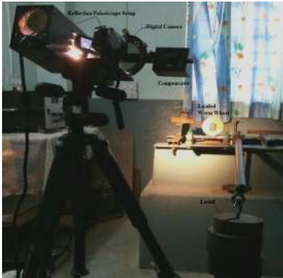
Fig -5: Experimental Setup with loading arrangement using Reflection Polariscope
