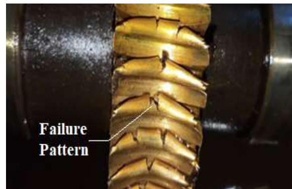
Fig -1: Damaged worm gear
