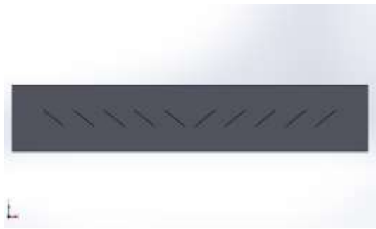
Fig.2- 24 Degree Louvered Fin in Design Modular
