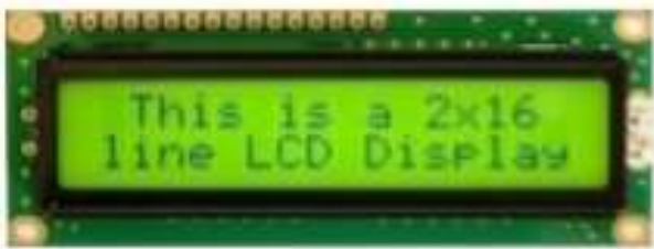
Fig 2: 16x2 character LCD display
