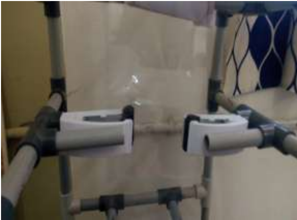
Fig-4.5: Vertical Sealing mechanism
