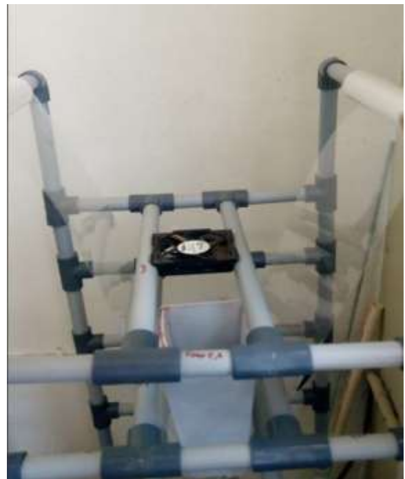
Fig 4.4: Packing Mechanism-Fan, Component collection box
