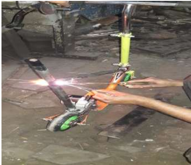
Fig -2: Arc Welding
