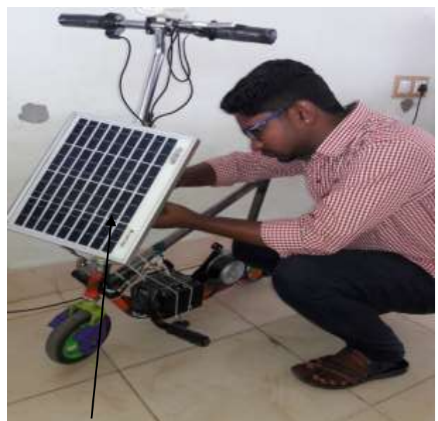
Fig-5: Solar panel
