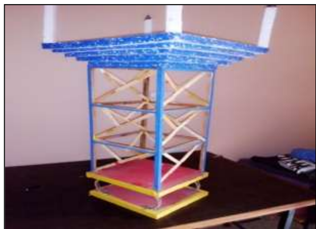
Fig 6: Model of Base Isolation with Spring as its base
