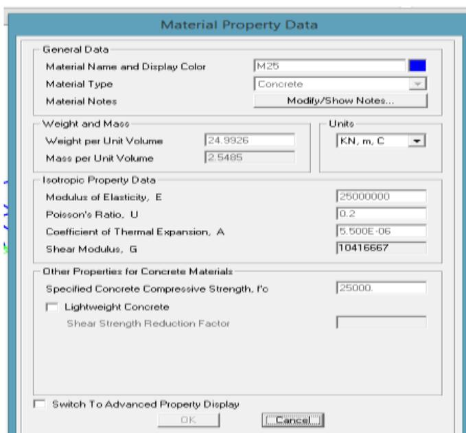
Figure 7: The material specifications for concrete grade M25
