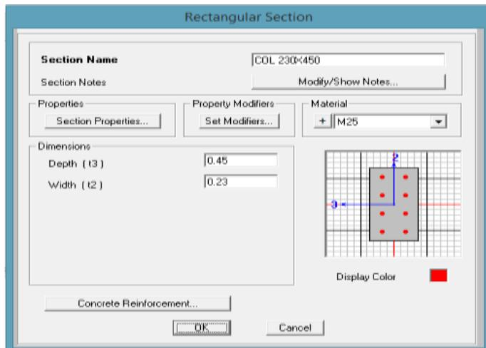
Figure 11: Column section details for all the columns in the structure
