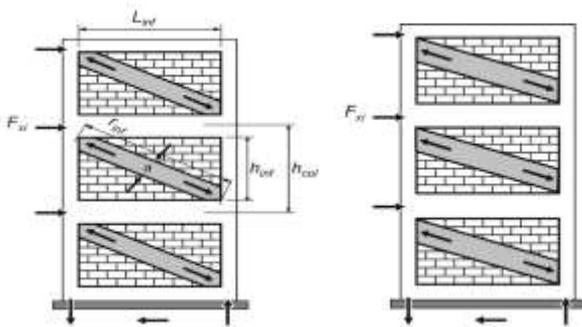
Figure 1: Concentric Struts      Figure 2: Eccentric Struts
