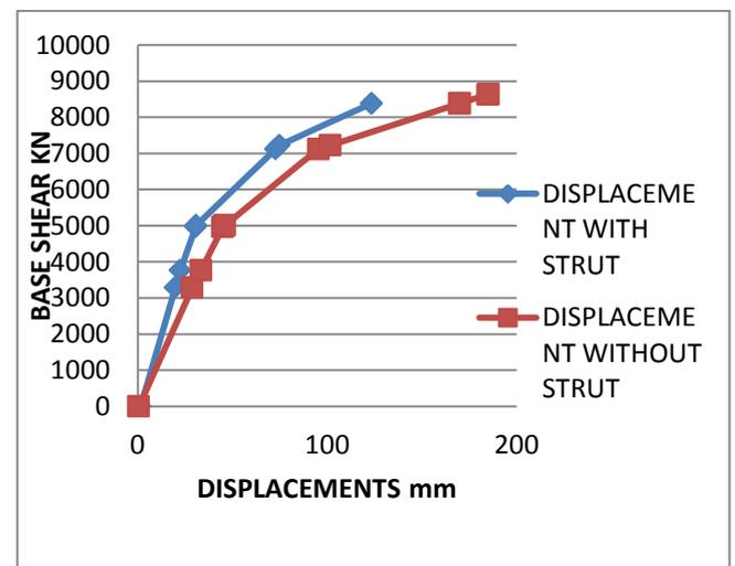
Graph 2: Base shear Vs Roof displacement curve for Building in X direction
