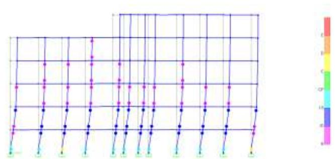
**Figure 18: Load Resisting Mechanism for a typical frame of Building for Bare Frame**
