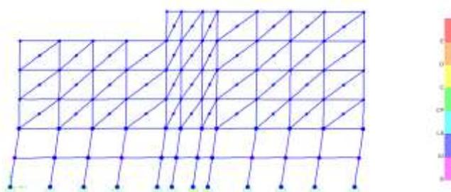
**Figure 17: Load Resisting Mechanism for a typical frame of Building with Infill panels**
