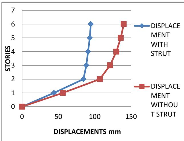
**Graph 4: Displacement profile of Building at the formation of mechanism in X direction**
