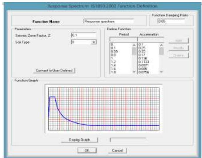
Figure 13: Response spectrum Function definition as per IS 1893-2002
