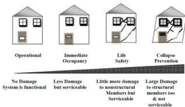
Figure 3: Performance levels and damage functions
