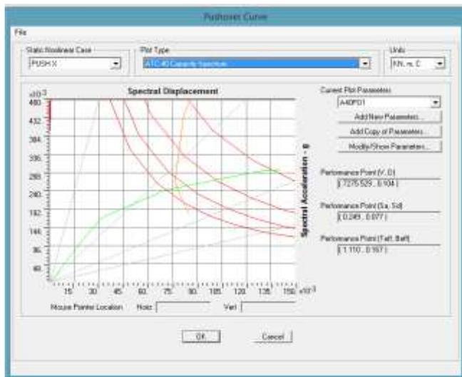
Figure 15: Capacity curve & Demand curve also Performance point
