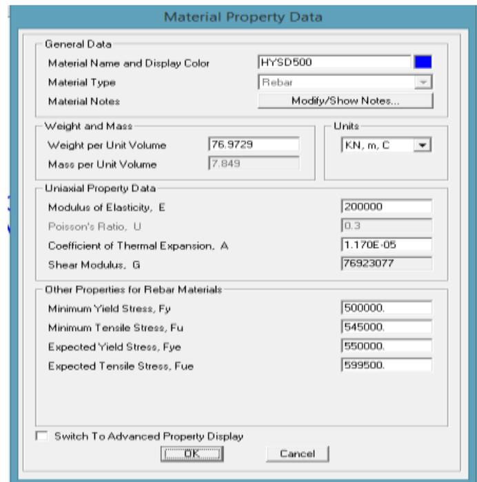
Figure 8: The Reinforcement grade specifications for HYSD 500
