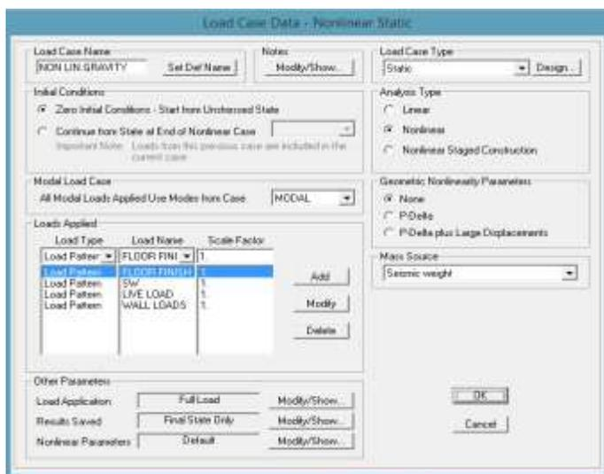
Figure 12: Non Linear Static load case for Gravity loads
