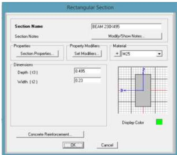
Figure 10: The Floor beams section details in the structure
