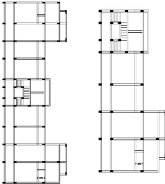
Figure 6: Framing Plans of all the floors
