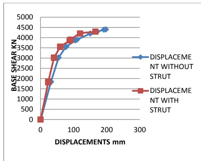
Graph 3: Base shear Vs Roof displacement curve for Building in Y direction
