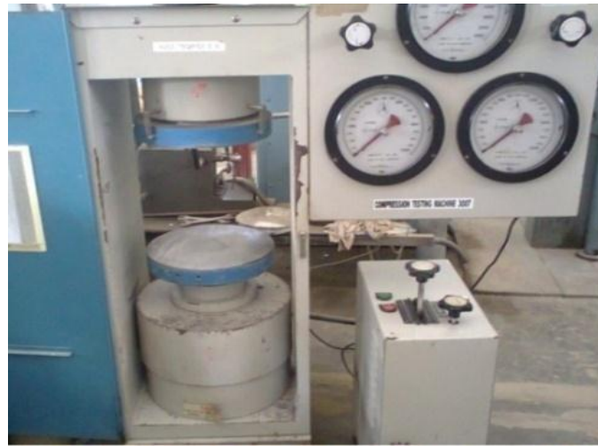
Fig. 3.8. Compressive strength apparatus
