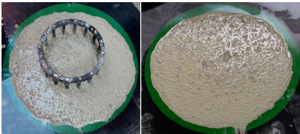
Fig. 4.1. Slump Flow Test Results
