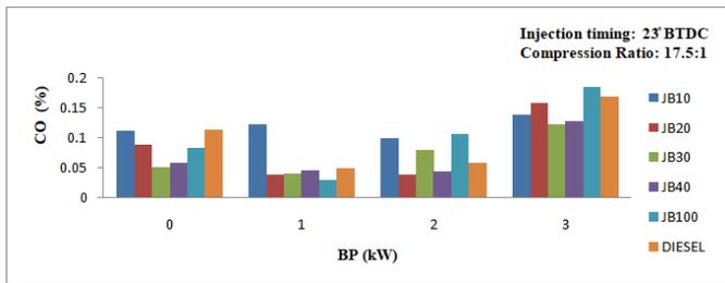
**Fig.3.7 Variation of CO emissions with respect to brake Power**
