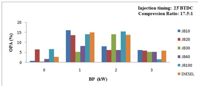
**Fig.3.8 Variation of OPA emissions with respect to Brake Power**
