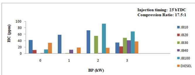
Fig.3.4 Variation of HC emissions with respect to brake Power
