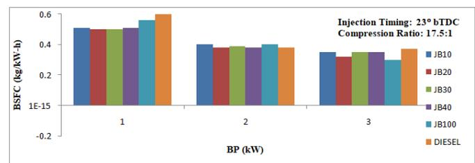
Fig.3.2 Variation of BSFC with respect to brake power
