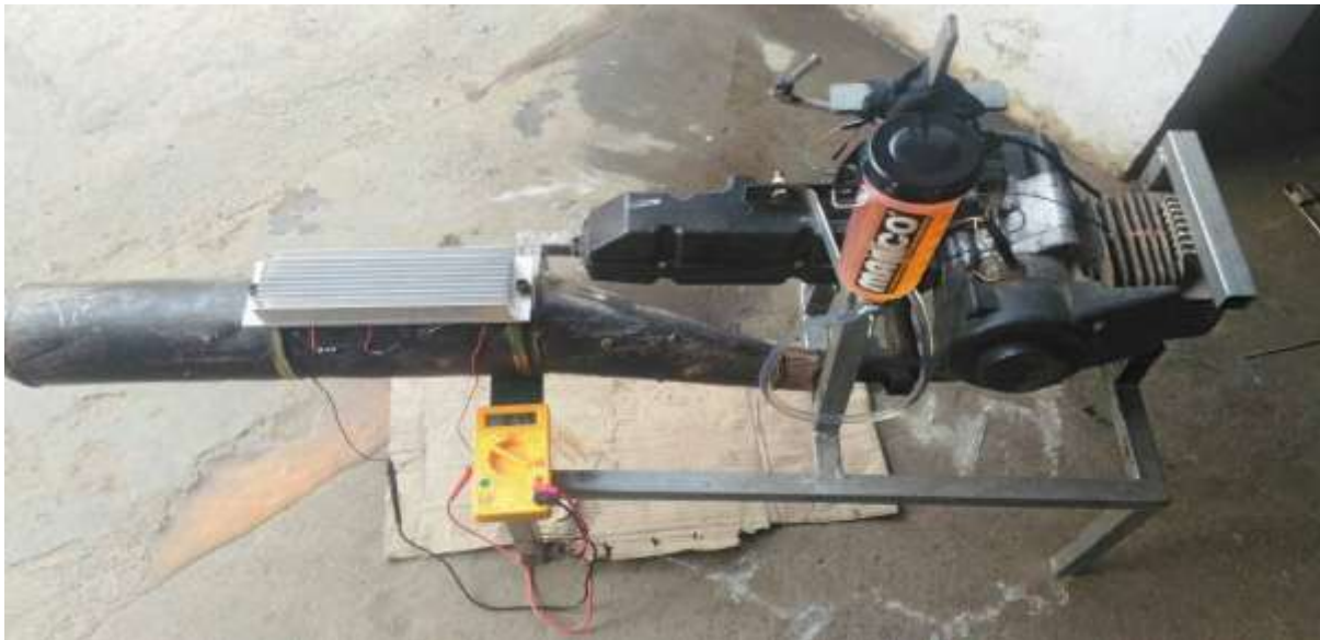
Fig 3.1: Experimental Setup with TEG Modules
