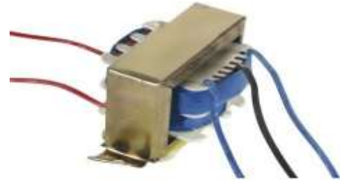
FIG3.3 An ELECTRICAL TRANSFORMER
