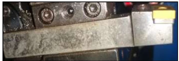
FIGURE.1 CNMG120408 insert (PVD) with Tool holder PCLNR 2525 M12
