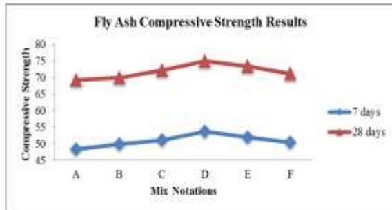
Compressive strength for Fly ash optimum dosage with different copper slag percentages
