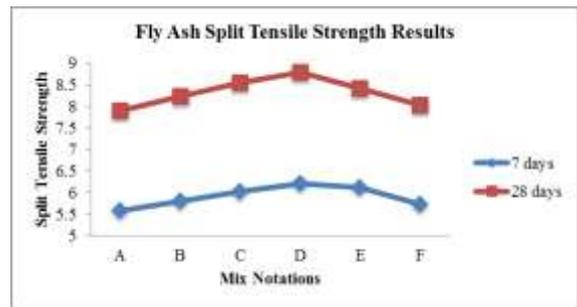
Tensile strength for Fly ash optimum dosage with different copper slag percentages
