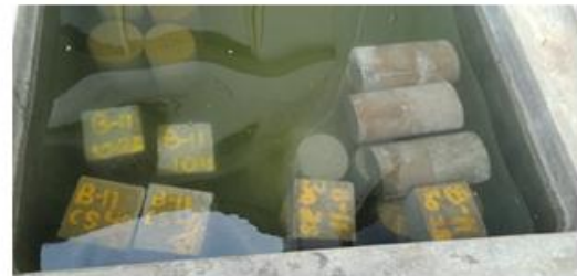
Fig -1: Curing Of Specimen
