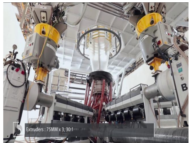
Fig- 2: Three-layer film extrusion system
