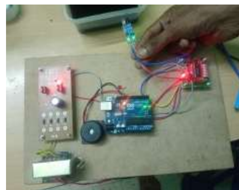
Fig 5.1 Transmitter Side prototype
