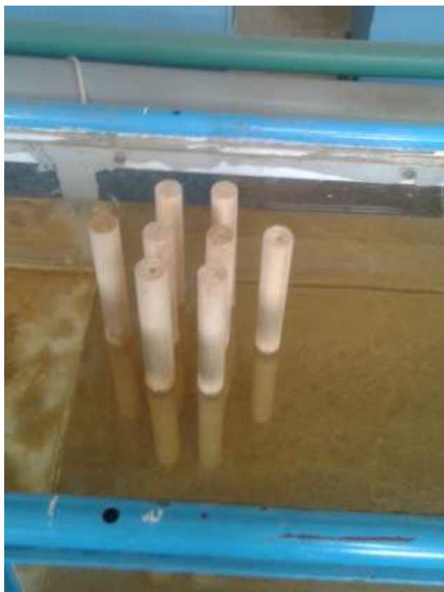
Figure (15) the effect of streamlined shape for piles
