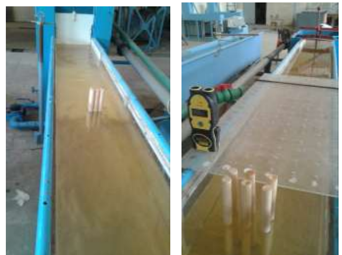
Figure (9) The wooden piles in the flume
