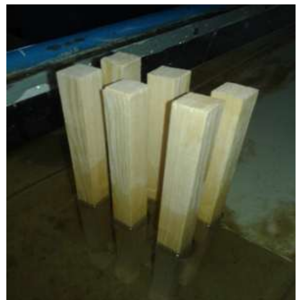
Figure (13) the bed profile around square piles before scour test
