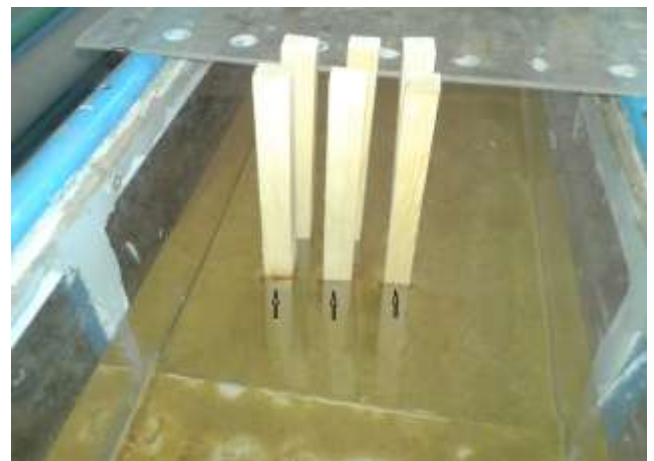
Figure (12) the bed profile around square piles after scour test
