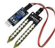
Fig-2: SOIL MOISTURE SENSOR
