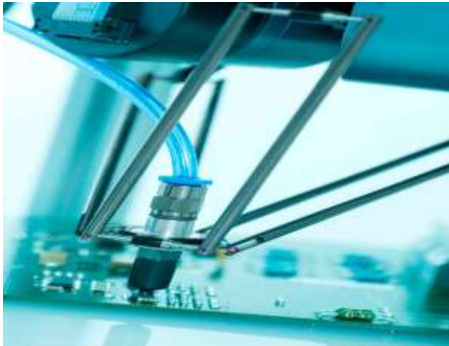
Fig – 6: Delta Robot Preparing Electronic Circuit Board [19]
