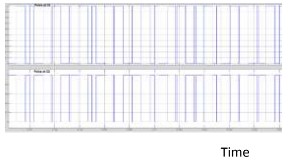
Fig 7: pulses from the PWM
