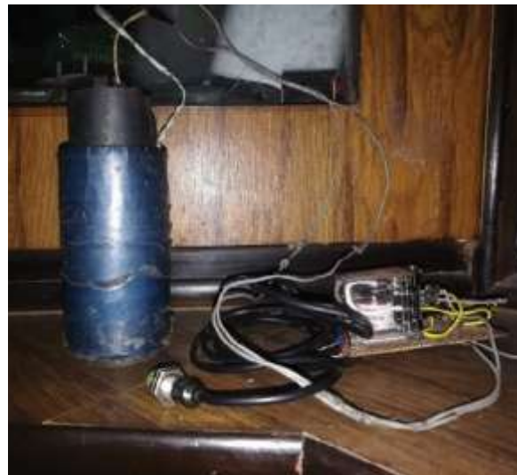
Figure 4: Electromagnet with Relay and Proxy Sensor
