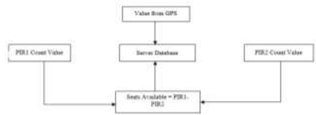
Fig - 2.2 PIR and GPS Sensor Data Collection
