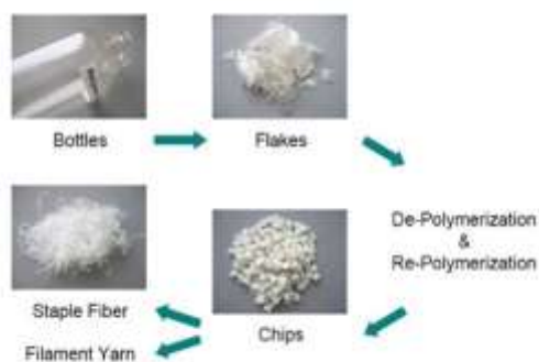
Fig -2(a): Preparation of fabric by recycling plastic
