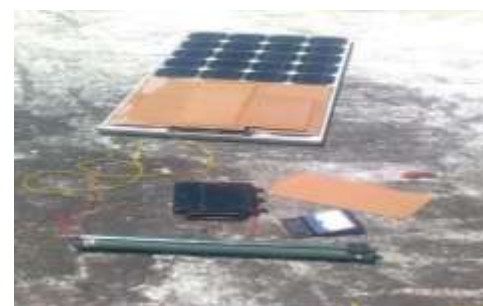
Fig - 2: Shadow by 1/2area of solar panel
