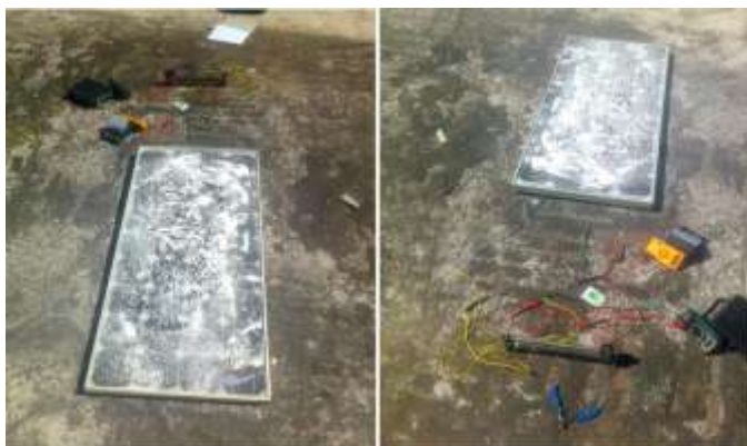
Fig - 4: Spread the 10g dust spread the 20g dust
