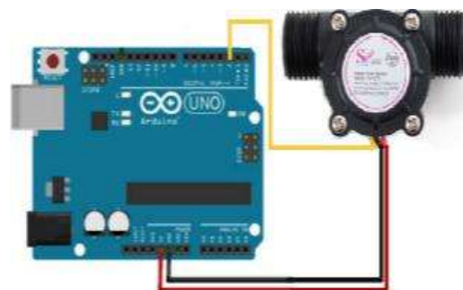
Fig 5.1: Interfacing of flow sensor with Arduino
