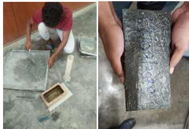
Fig 1: cement paver blocks preparation
