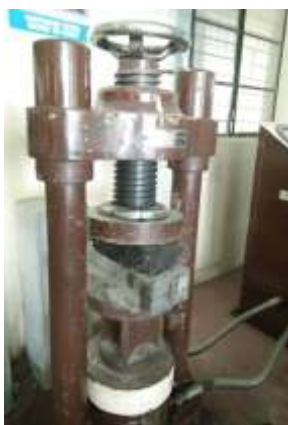
Fig-3: experimental setup for compression test
