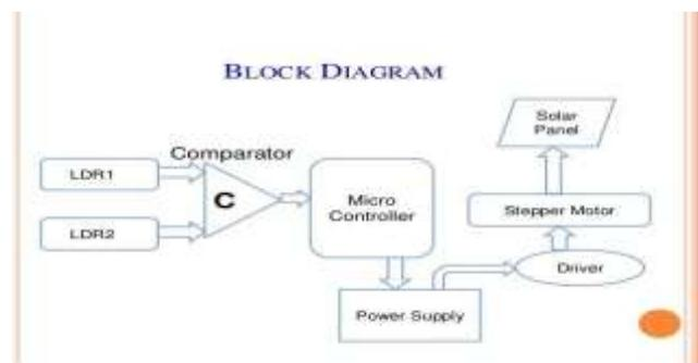
Fig. 1.1 Block Diagram of Dual Axis Solar Tracker
