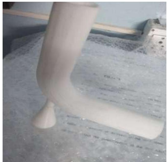
The above shown picture is our actual prototype model. This prototype is made up of PLA material (polyLactic acid) using the method of 3d printing.
