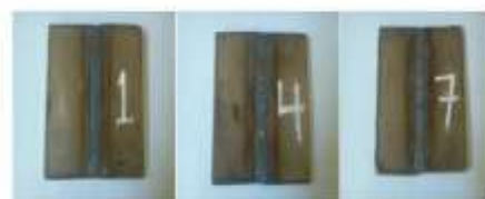
Fig.2.2: Specimen Of Mild Steel after welding
