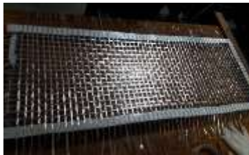
Fig.1. Formation of textile fibre grid
