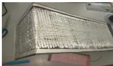
Fig.3. The fibre mat on the metal mould for resin application
