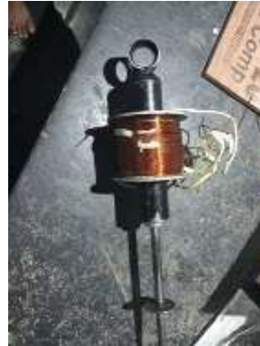
Fig -3: Structure of MRF damper
