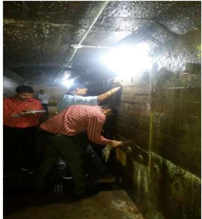
**Fig-2: Ultrasonic Pulse Velocity Test on Gallery of Dam**
