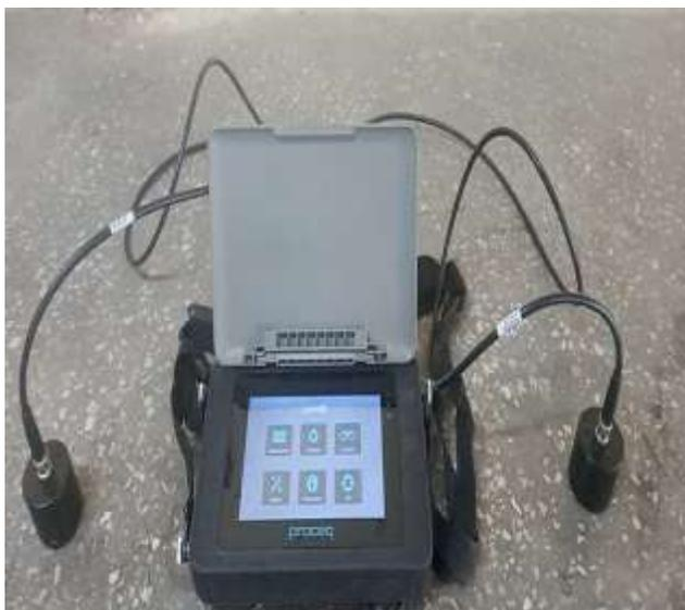
**Fig- 1: Ultrasonic Pulse Velocity Test Equipment (Proceq Model- PL 200)**
