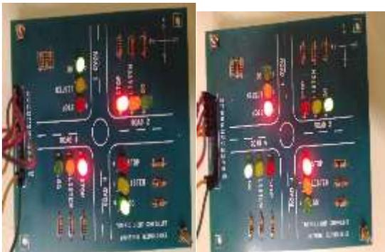
Fig.8 Output of Traffic Light Control on either direction of road
