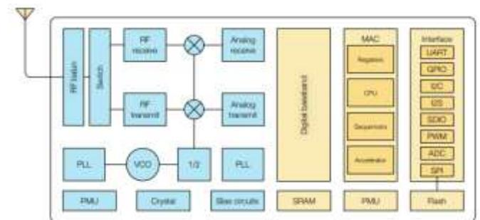
**Fig-2: ESP8266 block Diagram**
