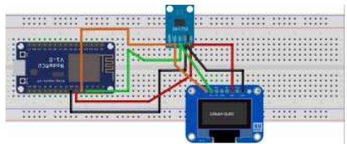
Fig-6: Connection with ESP8266
