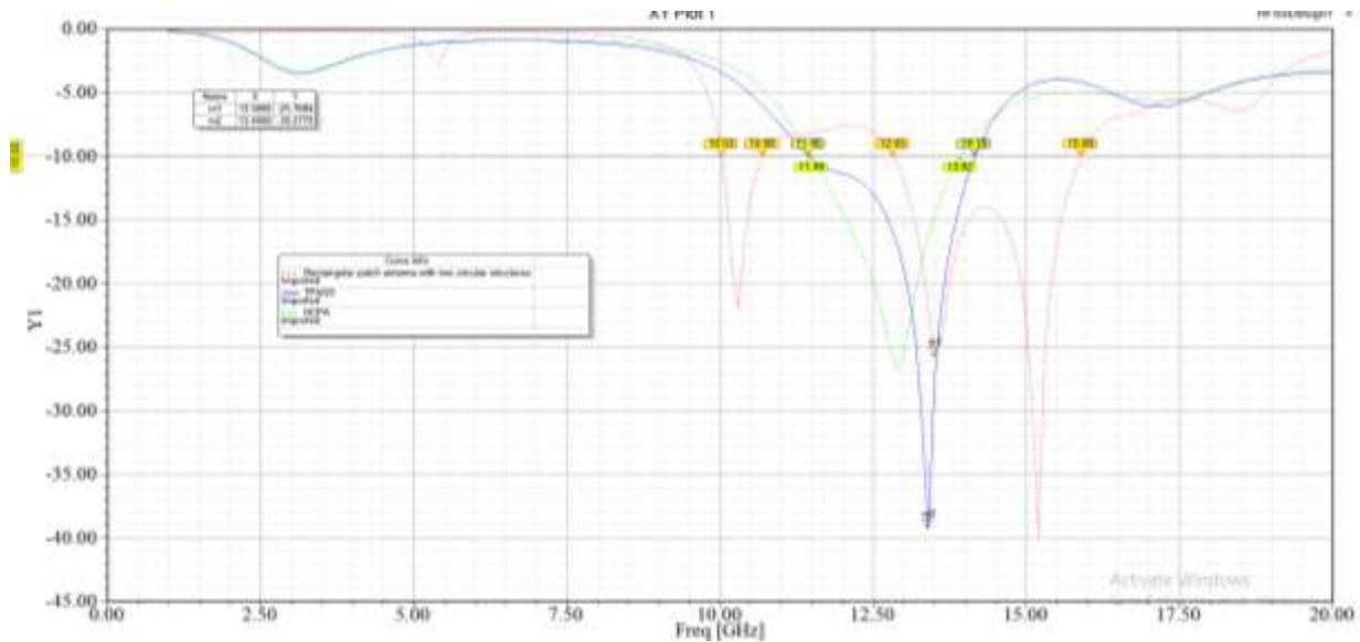
Fig 8: Return losses for the proposed antenna.
