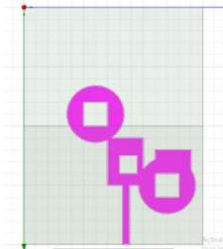
Fig 4: Actual design of the patch antenna
