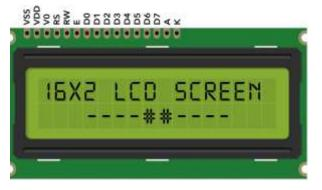
Fig -6: Liquid-Crystal Display
