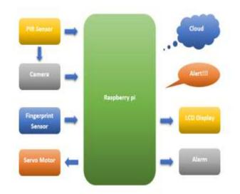
Fig -1: Block diagram of Proposed System
