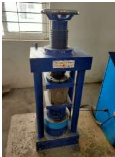
Fig -9: Compressive strength for Cube
