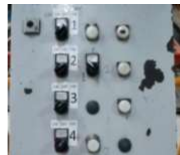
Fig -3: Tag replacement on the Control desk
