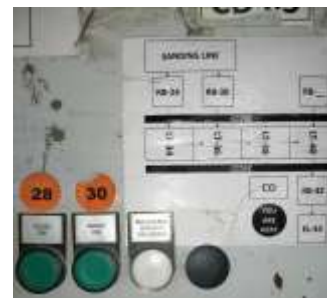
Fig -9: Control area Map is placed on CD at sanding line exit
