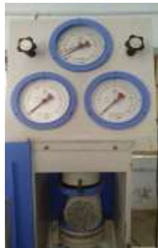
Fig 2:- Testing of Cylinders
