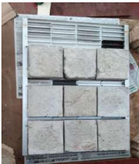
Fig - 2 : Adhesive kept for drying using clamping with dead weights
