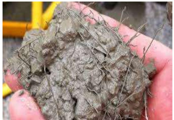
**Fig -1:** Steel Fiber Reinforced Concrete
