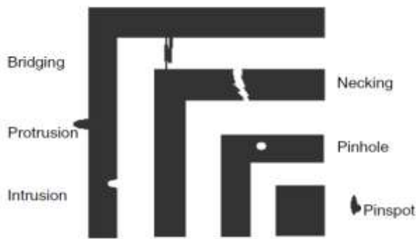
Fig. 4.4 Defect in photo mask
