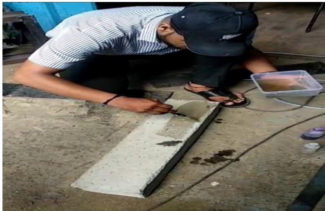
Fig -2: Application of Hakson’s High glass epoxy resin
