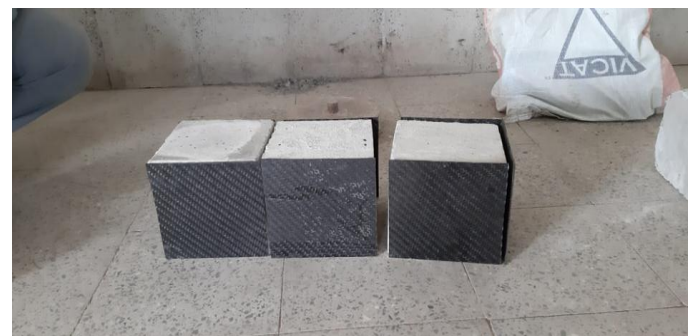
Fig -7: Application of CFS on the cube
