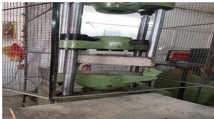
Fig -5: compressive testing
