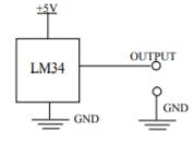
Fig 4:LM34 Interfacing Diagram
