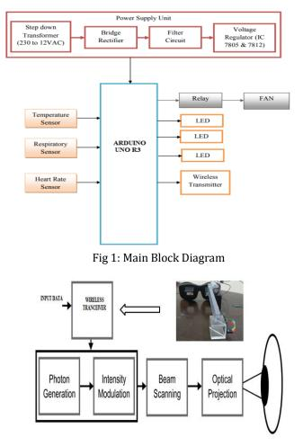
Fig 2: Functional Diagram for AR Glass
