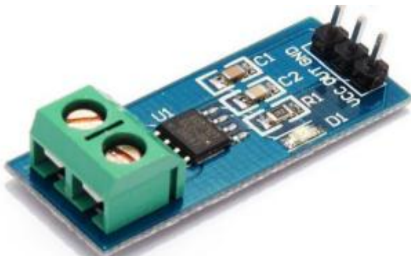
Fig.4.ACS712 Hall Effect Current sensor
