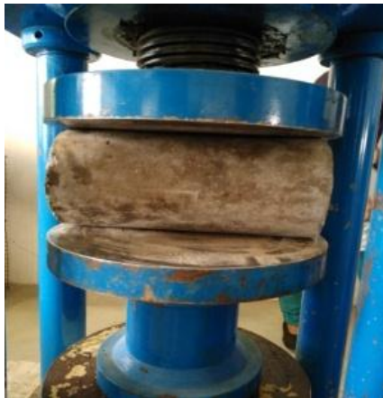
Fig -8: Split Tensile Strength Test
