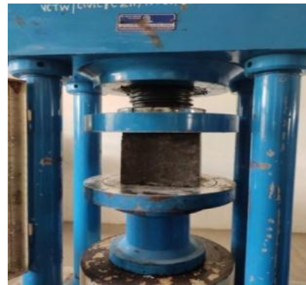
Fig -7: Compressive Strength Test
