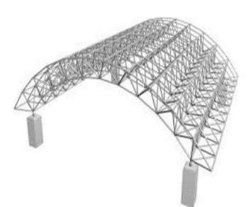
(b) Barrel Vault Space Structure
