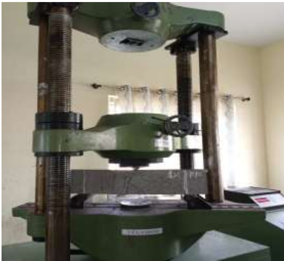
Fig-5.3: Flexural test on conventional concrete
