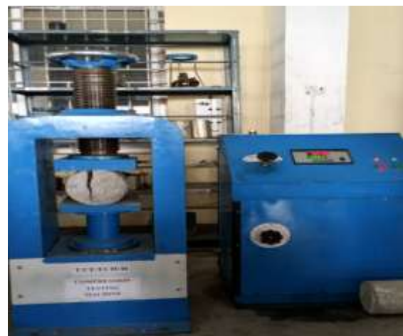
Fig-5.2: split tensile test specimens of conventional concrete prism
