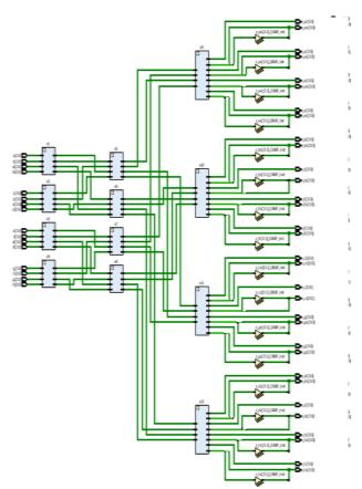
Fig 4.2 Schematic diagram of 8-point FFT using Compressor
