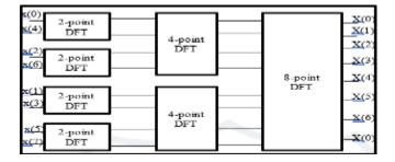
Fig :2.1 8-point Radix-2 FFT using Butterfly structure
