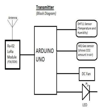
Fig -2: Transmitter side block diagram
