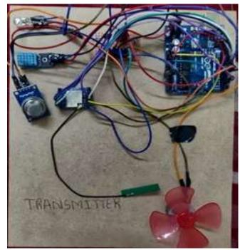
Fig -4: Transmitter side circuit
