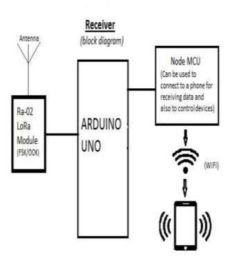
Fig -3: Receiver side Block diagram
